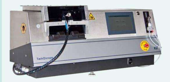
Rheology measurements are a major factor in the development and production of printing inks, raw materials for inks and other pasty liquids. Important factors for offset printing inks are tack (or stickiness of the ink), water pick-up, water release and viscosity.
