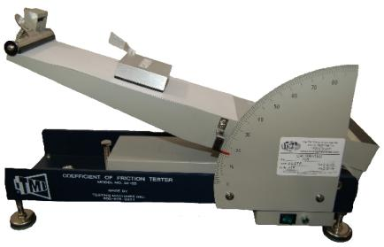
Slide Angle Friction is a measurement of a sheet like substrate such as paper, corrugated, plastic film or paperboard which determines the angle of inclination at which one substrate affixed to a sled will begin to slide/slip against another substrate of a similar material.
